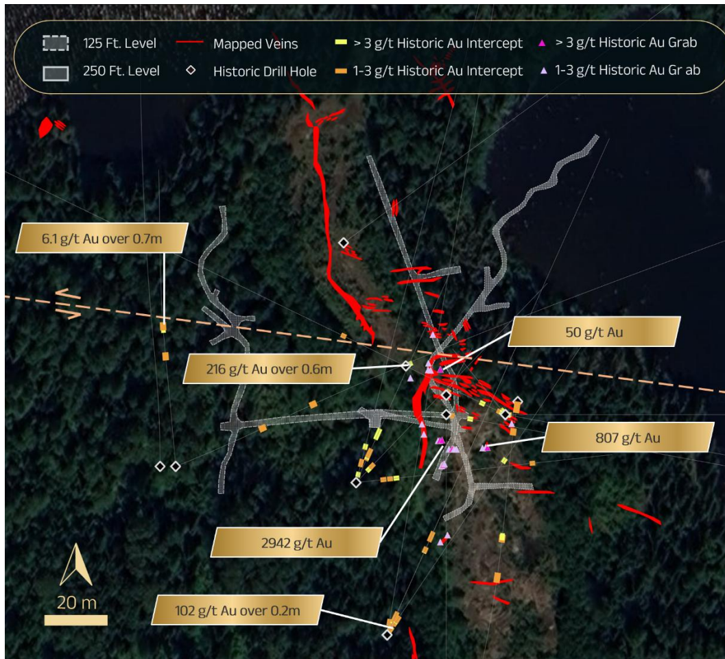
Figure 2: BobJo Project map showing vein trends, mapped veins, historic underground workings (125 ft and 250 ft levels), historic drill holes, and historic gold grab and intercept results.
